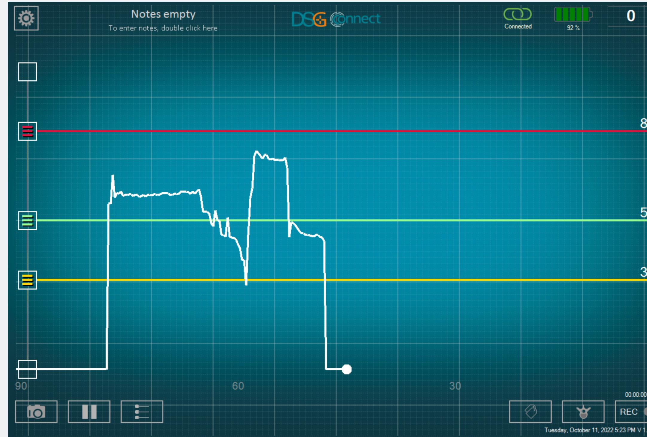
The reference lines feature allows you to position a landmark on the graph which you can adjust according to your drilling.
