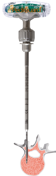
Fig. 14 Drilling through the pedicle
