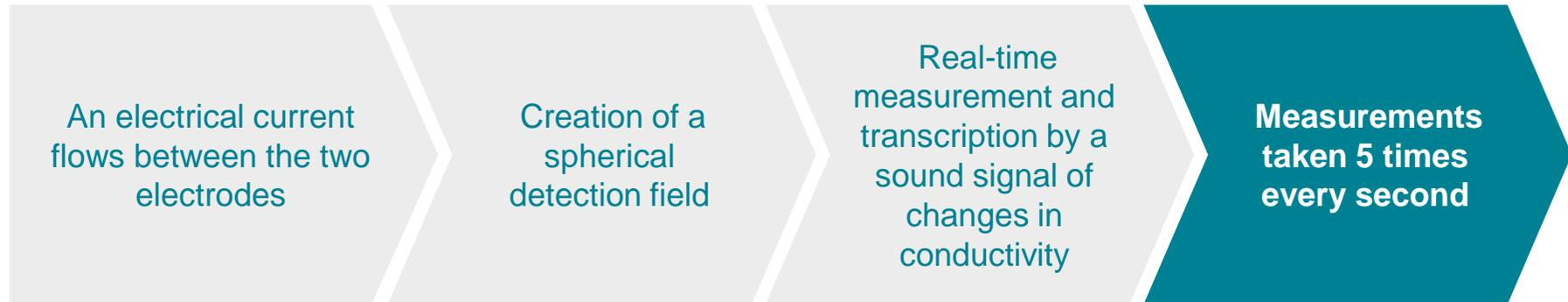
**The bipolar sensor: local measurement and transcription of electrical conductivity**
