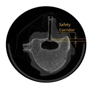
Example of the drilling accuracy, obtained via postexperiment micro-CT imaging
