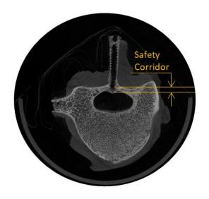
Example of the drilling accuracy, obtained via postexperiment micro-CT imaging. In 104 drillings performed robotically, the tip of the drill bit was automatically stopped at an average distance of 0.65mm from the bone limit.
